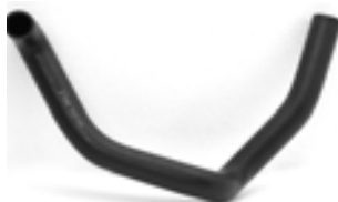
JKP Part No : R71672 Force motors - Tempo Traveller Radiator Bottom Hose ID = 36 mm, L = 920 mm
