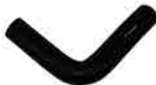
JKP Part No : R81202 Tafe Tractor - 241 DI L Type - Bottom ID - 38.1mm (1 1/2") L - 371mm (14 2/3")
