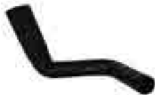
JKP Part No : R61274 TATA Motors - 1613 / 2515 Turbo Engine - Bend Hose ID = 44.5/58 mm [1 3/4"- 2 1/3"], L = 620 mm [24 1/2"]
